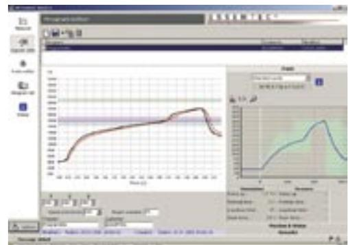
With RO-CONTROL new soldering tasks can be simulated and it offers unlimited storage space for programs. Measured temperature profiles can be superimposed graphically.
