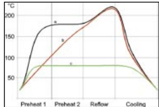
The perfect zone separation of the RO300FC allows the setup of profiles for all applications: a) lead free profile with soak platform, b) lead free profile without platform, c) curing profile for adhesives.
